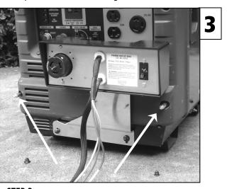
**STEP 3** Insert two standoffs into the two upper holes, and hand tighten.
